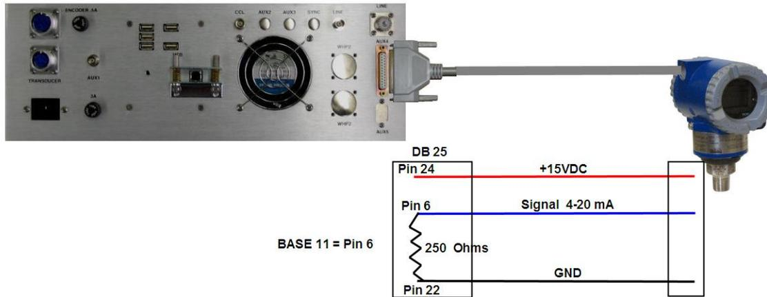
FIG: 13.21 AUX 4 Hardware Connections
